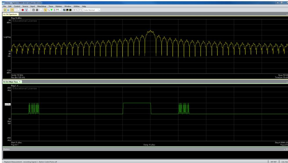
**Figure 3:** *The spectrum and phase of a pulse modulated with a Barker code.*
